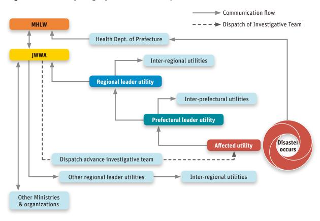
Figure 2.3 Water Utility Emergency Communication Flow upon Disaster
