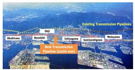
Figure 3.10 New Transmission Pipeline with Emergency Water Storage Capacity, Kobe City
