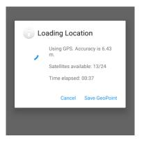
HDOP) provides a general indication of accuracy, though its reliability is disputed and should not be considered a precise measurement.
