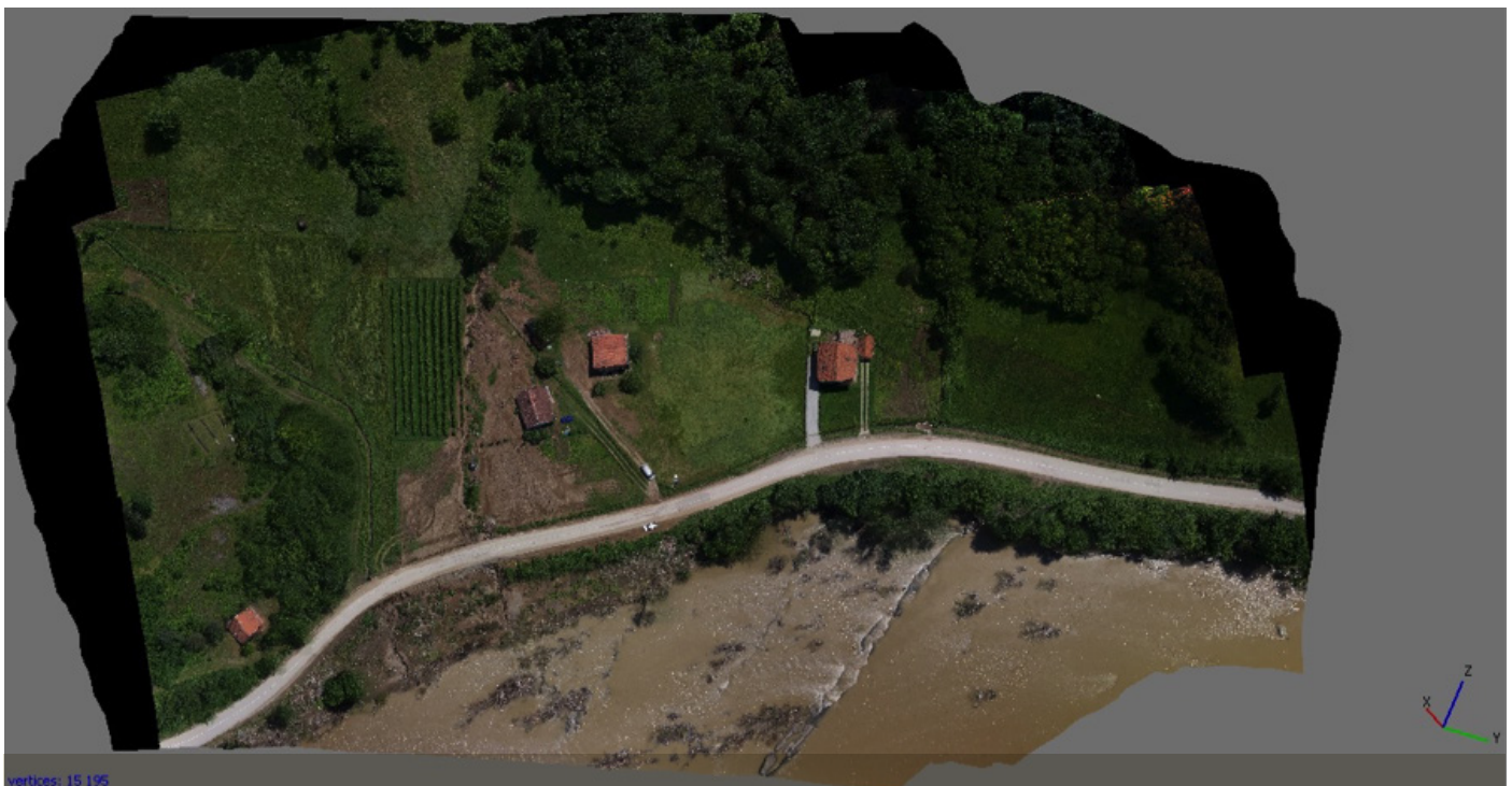
Figure 2 Example of a digital ortho-mosaic depicting a landslide that crosses a minefield in the upper part of the mosaic. The digital ortho-mosaic was derived from aerial images captured by UAVs.
