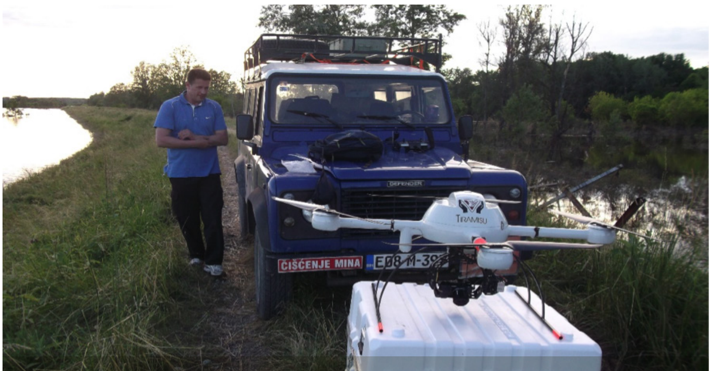
Figure 3 ICARUS and partners setting up their multi-rotor UAV to inspect flooding. © ICARUS.
